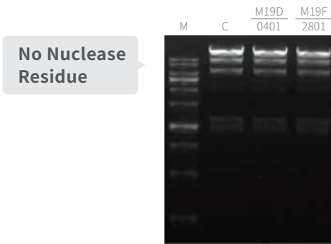
Figure. A 50 μL reaction containing 500 ng lambda DNA/Hind III and 200 U MRI is incubated at 37°C for 4 hours, the electrophoretic bands were consistent with the control.
