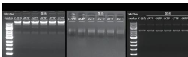
Fig. The detection results show that dNTPs have no DNase, RNase and Endonuclease.
