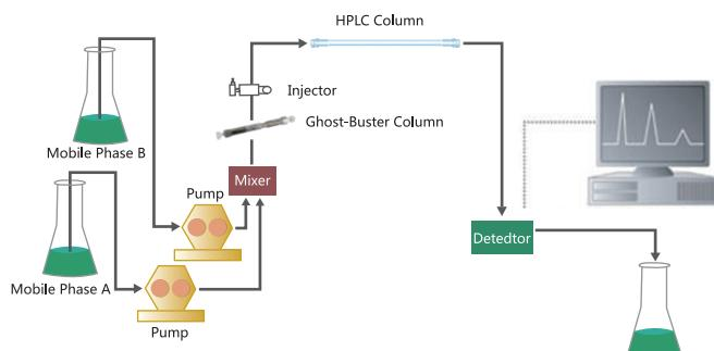
Installed between the gradient mixer and the sampler, Ghost-Buster column can trap most ghost peaks before HPLC analysis.
