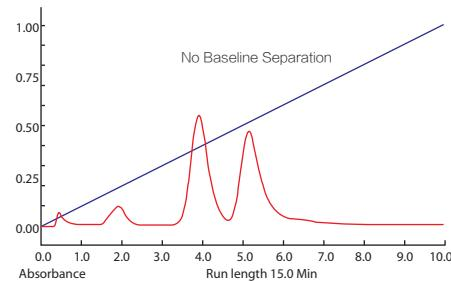
WelFlash Column: 4 g Amorphous Silica (40-63 µm)
